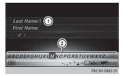
In the example, a new entry is added to the phone book ( $\triangleright$  page 102). The new entry has three input lines for entering the last name, first name and phone number. The input line for the surname is selected automatically.
