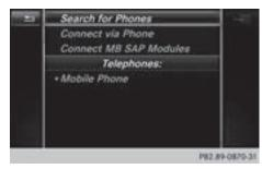
To select a mobile phone from the device list: turn the controller and press to confirm. If the mobile phone supports the Bluetooth<sup>®</sup> PAN profile, Internet access is set up. You can use the Internet functions.
