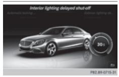
The interior lighting is activated for the duration of the switch-off delay time when the SmartKey is removed from the ignition lock.
