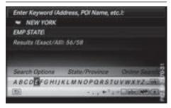
The keyword search is used to help find destinations using fragments of words. The keyword search is tolerant of errors.
